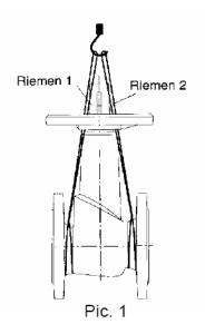
The lifting belts 1 und 2 must be twisted round the body. In order to keep the valve in the shown position and to prevent falling vertically, the two lifting belts should lead to the hook through the handwheel arms.
